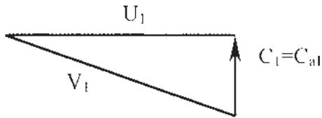
**Figure 4.15** The velocity triangle at the impeller eye.
