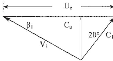
**Figure 4.16** The velocity triangle at the impeller eye.
