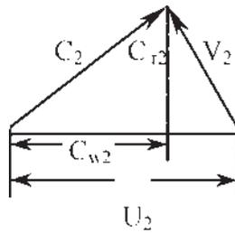
**Figure 4.12** Velocity triangle at the impeller tip.
