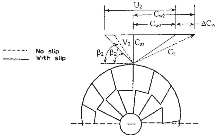
**Figure 4.6** Centrifugal compressor impeller with radial vanes.
